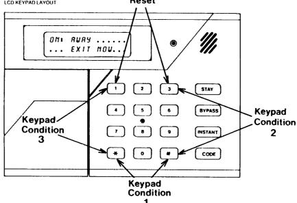
The keypad emergency conditions are programmable and can be used for conditions such as PANIC, FIRE, MEDICAL, AUX, etc. These special zones can duplicate existing hardwired zones.
